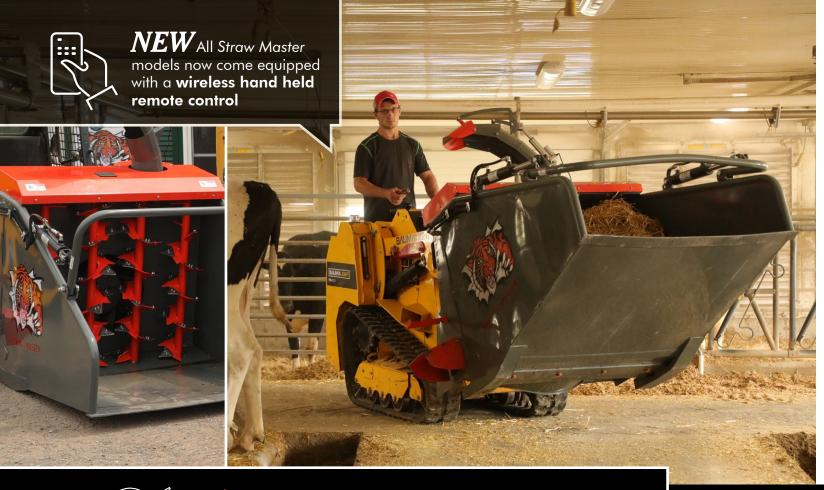
The Straw Master Round features the same narrow design as all Straw Masters, while delivering flexible amount of bale types and sizes. This machine will accommodate 4'x4' and 3'x4' square bales, and round bales up to 4'x 5'. With full vibrating floor, this machine delivers smooth and steady feed in round bales with no apron chain or moving parts to break or fail.
