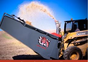
300 degree hood rotate allows you to spread on either side of the skid steer
